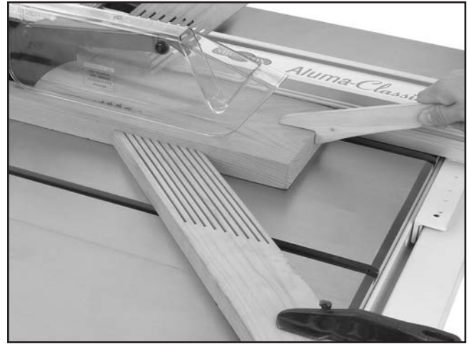
Figure 55. Typical ripping operation.
