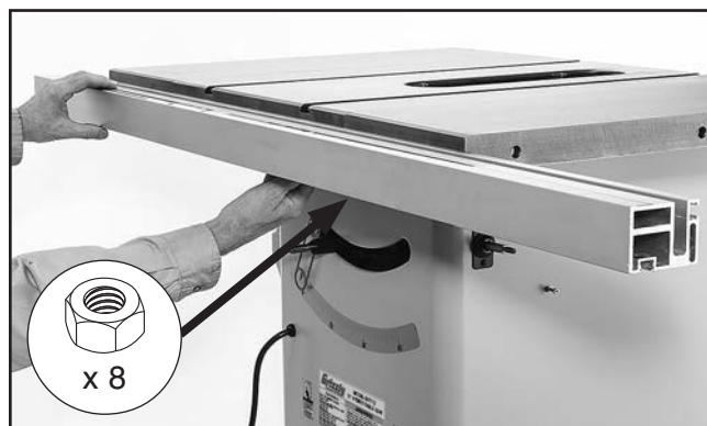
Figure 22. Mounting front fence rail.
