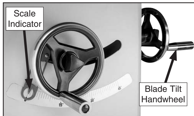
Figure 30. Blade tilt handwheel and angle scale.
