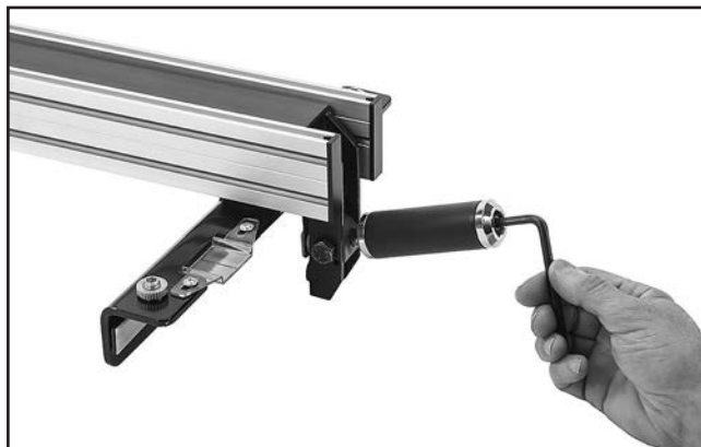
Figure 28. Installing fence handle.
