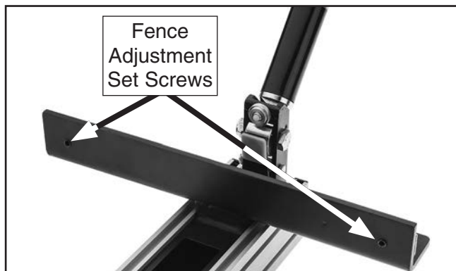
Figure 124. Location of set screws to adjust fence parallelism (shown upside down).
