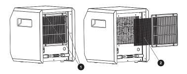
**CLEANING: CAUTION – Before cleaning the heater be sure to disconnect power cord and allow the heater to cool completely.** This heater should be cleaned at least once a year to maintain proper performance. Clean the outside surface with a clean damp cloth. Do not use harsh chemical or abrasive cleaners. DO NOT IMMERSE THE HEATER IN WATER. Allow heater to dry completely before use.
