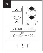
To view the ambient temperature press the ambient temperature button on the control panel.
