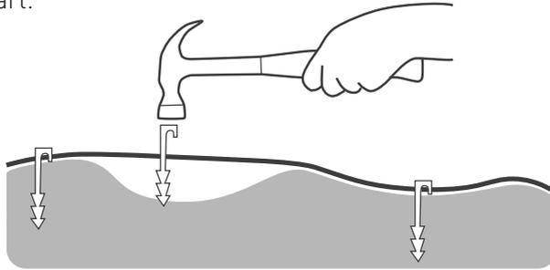
Hammer the extension cable into the ground so it's not a tripping hazard.
