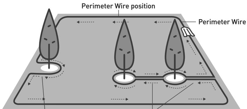
If the distance between an island and the perimeter wire is lower than 1.5 m [5 ft], make the obstacle part of lawn's edge.
