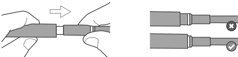
Connect the Power Supply unit to a regular power outlet.
