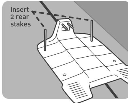
Be careful not to damage irrigation pipes when hammering down the stakes.
