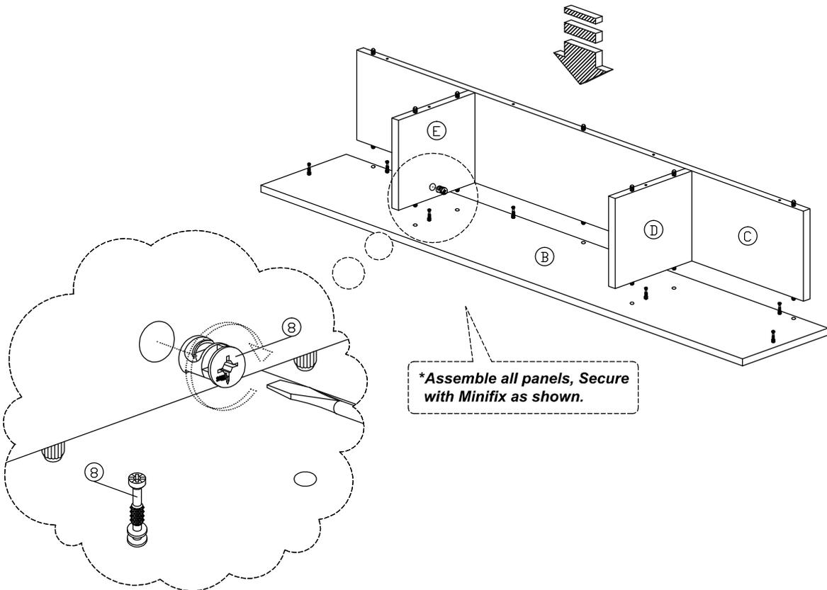
*\*Assemble all panels, Secure with Minifix as shown.*
