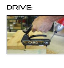
With the Marksman Pro-X1 set on the board, place one CAMO Hidden Fastener into the Screw Guides on both ends of the Marksman Pro-X1 tool. Note: if the tool is not set on the deckboard, the screws will slide out of the Screw Guides.
