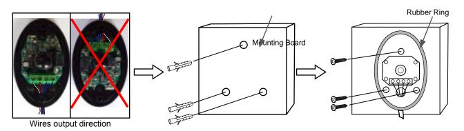
**Note:** With strong power, the PBS Switch may fail if the receiver is too close to the emitter. Take the receiver at least 1m away from the emitter and try again. Remove the condenser lens in both emitter and receiver if the distance is too close and the PBS Switch is not so sensitive. The PBS Switch should be sheltered from direct sunlight.
