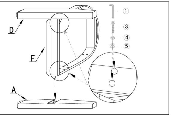
Install the Left Front Leg (A) and the Right Front Leg (D) onto the Seat cushion (F) connecting them via the Wooden Tenons (6), then using the Allen Wrench(1), Long Bolts(3), Spring Washers(4), and Flat Washers(⑤), attach them as shown in the picture above.
