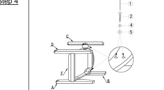
Install the Left Hind Leg(B) and Right Hind Leg(C) onto the Seat Cushion (F) using the Allen Wrench (①), Short Bolts(②), Spring Washers(④), and Flat Washers (⑤) as pictured above.
