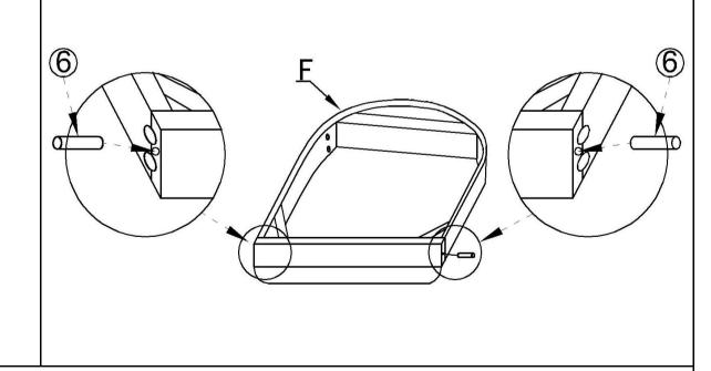
Install the Wooden Tenons(6) into the sides of the Seat cushion(F) as pictured above.
