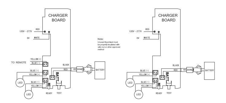
Note for HO models: Use 18-22 AWG stranded wire to connect remote lamp heads.
