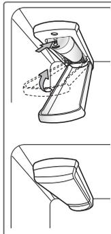
3 After the water filter is replaced, dispense 2.5 gallons of water (flush for approximately 5 minutes) to remove trapped air and contaminants from the system. Do not dispense the entire 2.5 gallon amount continuously. Depress and release the dispenser pad for cycles of 30 seconds ON and 60 seconds OFF.
