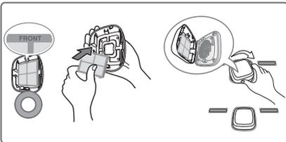
After changing the filter, push and hold the Fresh Air Filter button for three seconds to reset the filter sensor.
