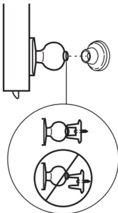
Place bumper assembly on wall so the door handle hits the rubber properly; if you have a button type lock, be sure button does not contact rubber to avoid accidental locking. Mark position of screw with a pencil through the center hole. If using a plastic anchor, pre-drill a 7/32" hole and tap in anchor; if using screw only, pre-drill a 1/8" hole; place assembly into position and install screw.
