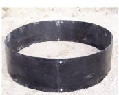
**Step 4**: Assemble the steel ring. Place the ring on the ground and using the bolts provided, bolt the two sides of the ring together. Install approximately 2" of clean porous rock or gravel inside the fire pit. Set the ring in the center of the blocks. Once the ring and blocks are all in place remove one block at a time from the top course and glue to the two blocks below using a quarter sized dab of concrete adhesive.
