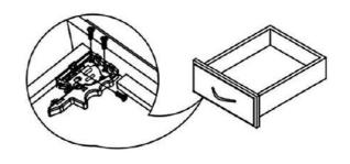
3 ) Please put the drawer flat on the slide, and close the drawer completely. When the slide be connected with the locking brackets, then the installation to be finished.
