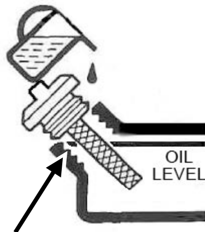
Figure 2 - Add Oil To TOP Of Threads
