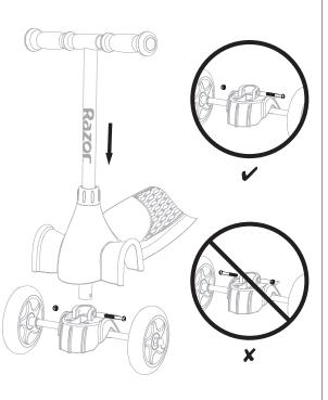
A warning: Failure to properly engage the spring-loaded buttons may cause the handlebars to dislodge while riding and may cause rider to lose control and fall. When correctly engaged, the handlebars will not rotate nor move sideways, and the spring-loaded buttons will be clearly visible in the holes on the T-bar.
