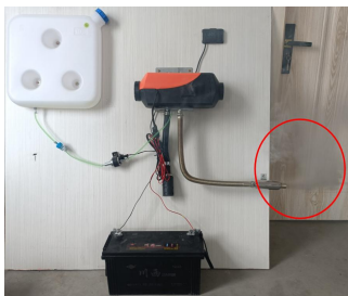
Excessive pump oil produces white smoke
