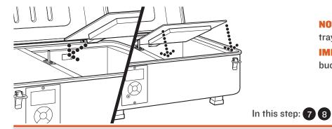
**NOTE:** Be sure the grease drain spout on the grease drip tray extends through the opening in the back of the grill.
