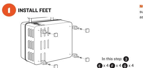
**NOTE:** You should assemble grill on a clean, flat surface, as you will need to lay it on its back during assembly.
