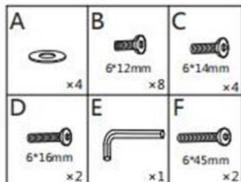
**STEP 1** ③ and ④ are connected to ⑤ respectively, ⑥ is connected to ③ and ④, B is inserted into the corresponding hole and fastened with E.
