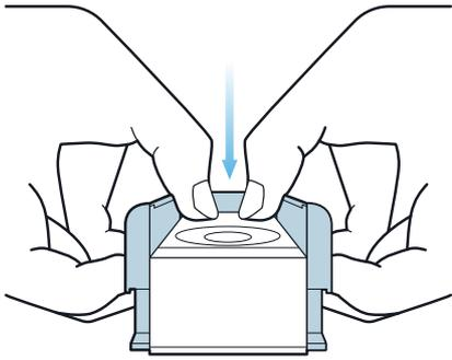
**A** Place your fingers in the indentations on the sides of the doorbell, simultaneously pull away and push the faceplate out.
