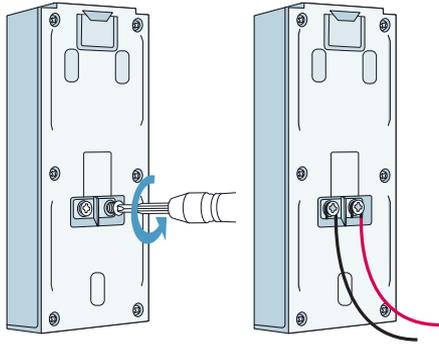
Loosen the terminal screws located on the back of your Wi-Fi Doorbell using the included Phillips head screwdriver. Place your existing doorbell wiring underneath the terminal screws, then re-tighten the terminal screws to secure the wires.
