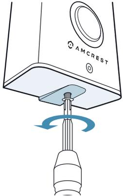
**B** Use the included Philips head screwdriver to remove the bracket screw from the doorbell.
