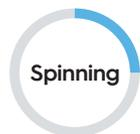
A spinning LED indicates the Wi-Fi doorbell is in setup mode and is currently not connected to a network. Please follow the installation instructions in the Amcrest Smart Home app to continue.
