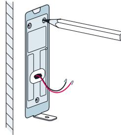
**B** Place the doorbell bracket to fit your existing doorbell wiring. Then mark the drill holes with a marker.
