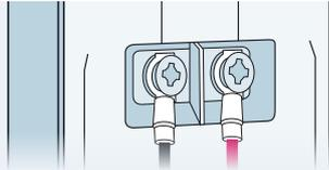
**NOTE** If your existing doorbell wiring is too short, use the included extra wires and wire nuts to extend your wiring. Remove the terminal screws completely then thread the screws through the extra wire.
