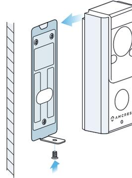
Feed the wiring back into the wall. Then, secure the doorbell to the mounting bracket using the included screwdriver.
