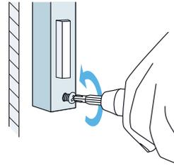
**A** Remove your existing doorbell from the wall and disconnect the wires. These are the wires we will be using to install your new Amcrest Wi-Fi Doorbell.
