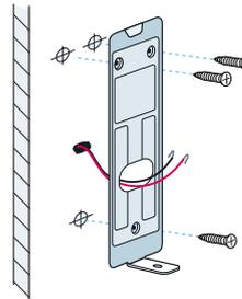
**C For Wood, Drywall or Soft Surfaces:** Secure the doorbell bracket to the mounting surface using the included screwdriver and mounting screws.
