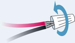
**NOTE** To attach the wires, align the ends of the two wires, place the wire nut over the exposed wiring and twist the wire nut clockwise to tighten.
