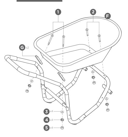
Attach the part F tray to the part B front frame with two part 2 bolts, two part 3 washers, two part 4 spring washers, and two part 5 nuts.
