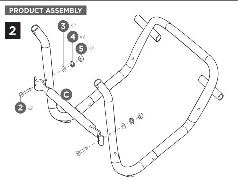
Attach part C center support with two part 2 bolts, two part 3 washers, two part 4 spring washers, and two part 5 nuts.
