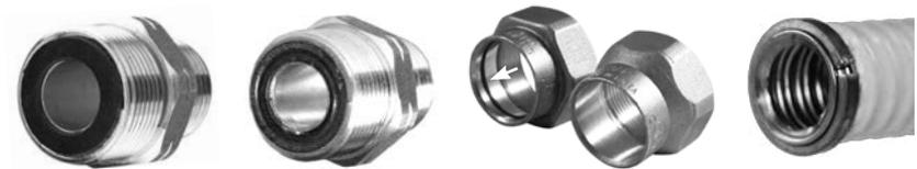
Figure 4.2 (1) Gasket in Fitting Before Assembly, (2) After Assembly (note groove in gasket), (3) Fitting with and without o-ring; and (4) Compressed Tubing
