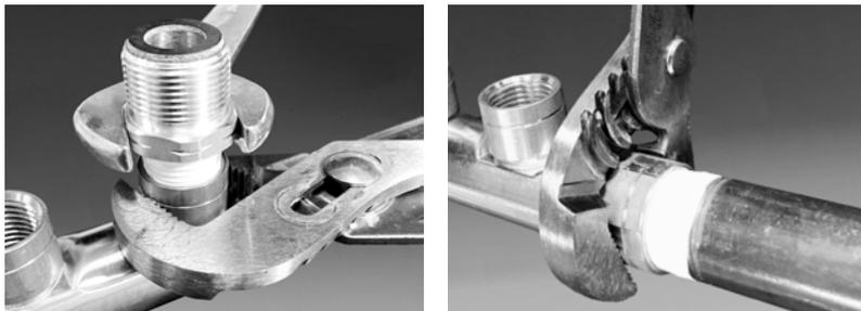
Figure 4.3 Supporting Manifold When Attaching Fittings
