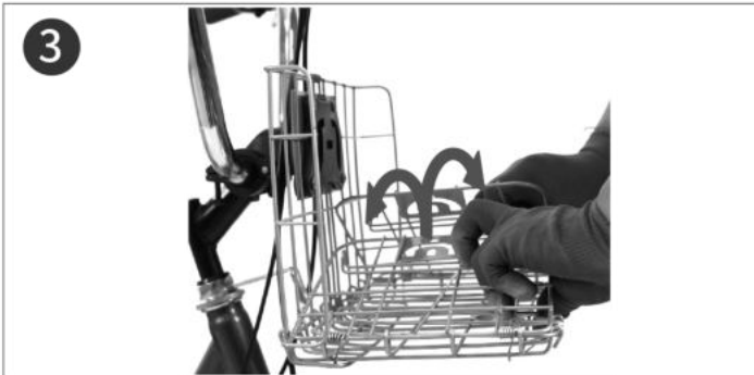
1. Place the front basket in the butt piece under the handle.
