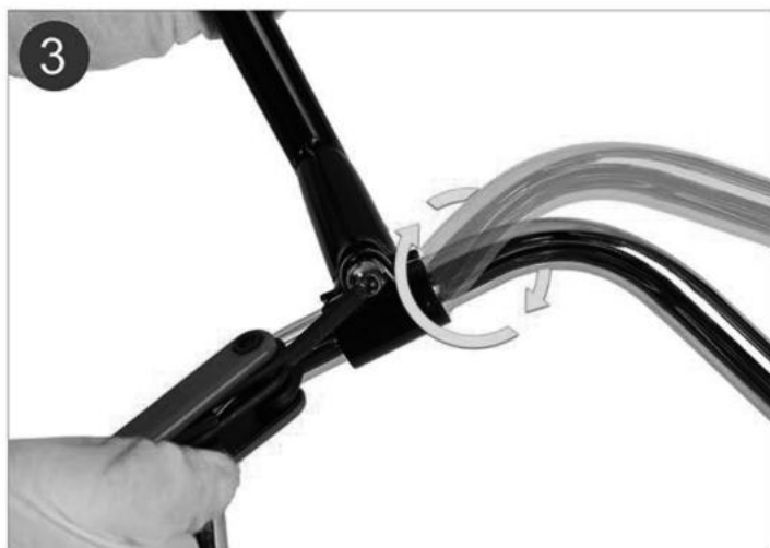
3. The screw here controls the angle of the handlebar. Please adjust the handlebar to parallel with the ground
