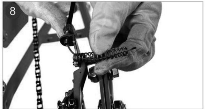
8. Put on the brake spring.
