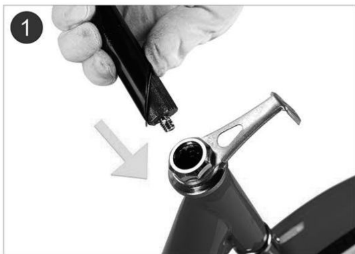
1. Insert the stem on the handlebar into the head tube.
