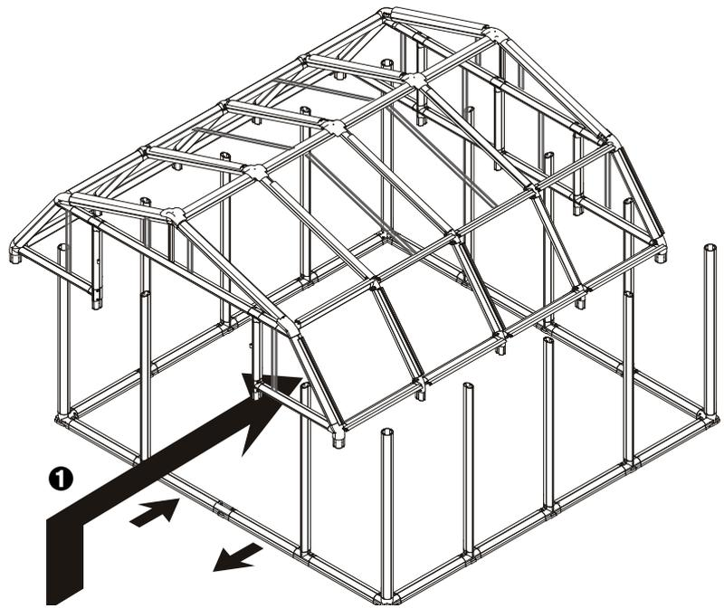
❷ Place the roof on the columns and circle around the greenhouse and insert the first 1 cm (1/2") of the roof connectors into the columns.
