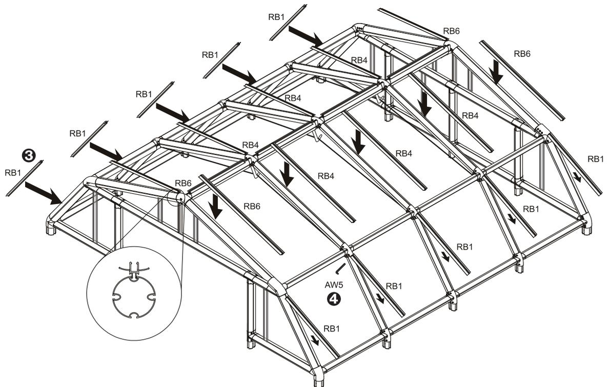
**Note:** If you have difficulty inserting the top of the RB1 glazing element slightly loosen the AS70 screw holding in the CAB40 cable.
