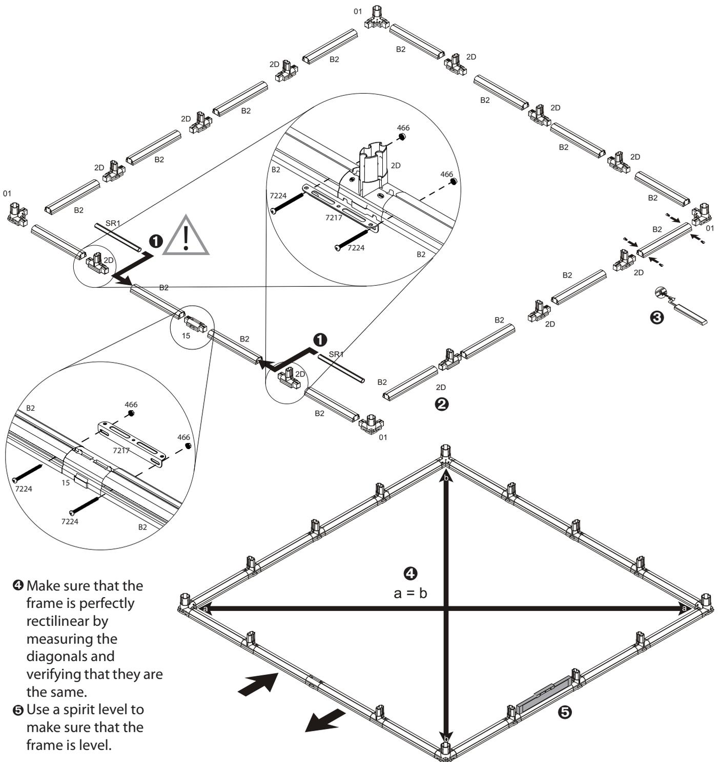
❹ Make sure that the frame is perfectly rectilinear by measuring the diagonals and verifying that they are the same.
