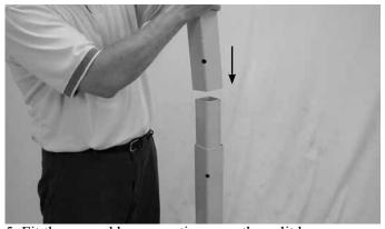
5. Fit the second boom section over the split boom connector. Align the corner access holes with those of the lower section.
