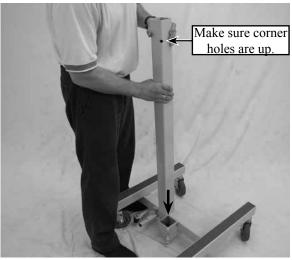
1. Install either of the boom sections into the dolly base. Make sure the holes in the corner of the tube are up.
