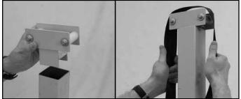
7. Insert the top roller assembly then position the strap over the top rollers, raising the Collar up the Boom.
