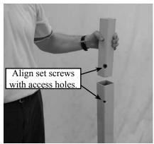
4. Insert the split boon connector. Align the set screws with the access holes in the boom tube
