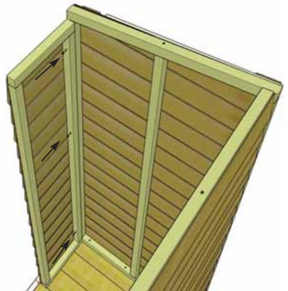
**12.** Align butt or bottom of wall siding flush with outside of floor framing. When correctly positioned, secure bottom wall plate to floor with 2 - 2 1/2" Screws (C). Attach vertical wall framings together at top, middle and bottom with 3 - 3" Screws (B).
