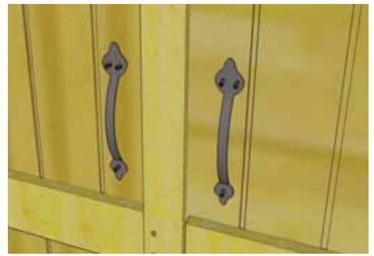
**46.** Attach **Door Handles (X)** to doors with **3 - 3/4" Black Headed Screws (J)** per handle. Choose desired handle height. Make sure screws go into interior door framing and are not exposed on inside.
