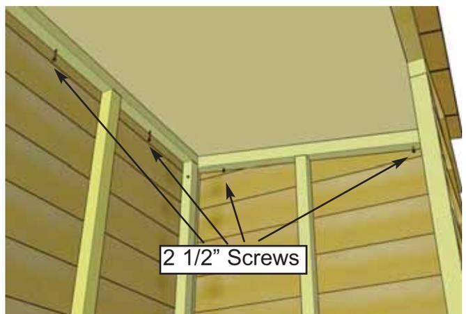
**27.** From inside the shed, start securing the roof by screwing the door header into Roof Panel on an angle with **3 - 2 1/2" Screws (C)**. Make sure screw tips do not go completely through roof panel. On the sides and rear, screw from upper framing into Roof Panel. Use 2 screws per each wall panel. Screw on an angle and make sure screw tips do not go completely through roof panel.
