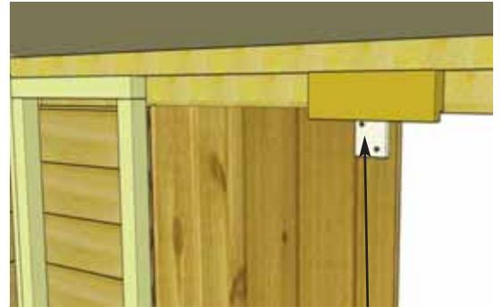
**48.** Install the **Barrel Bolt Plywood Spacer (UU)** to interior door frame, flush at the bottom, and 1/4" from edge, as pictured. Use **2 - 1 1/4" Screws (E)** to secure.
