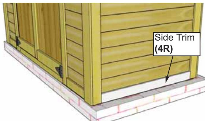
**44.** Attach both **Lower Side Narrow Trims (4R)** ( $1/2'' \times 2 \ 1/2'' \times 31''$ ). Place trims between front and rear corner trims to cover part of floor frame with **4 - 1 1/2'' Finishing Nails (K)**.
