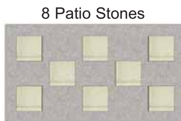
Gravel Foundation with Patio Pavers
