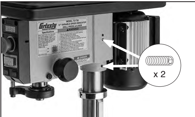
Figure 12. Location of set screws that secure headstock to column.
