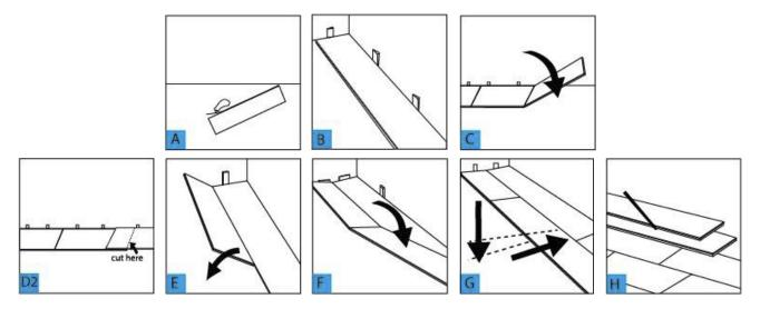
Always check flooring planks for defects such as chips and color variations under good light conditions. Check that grooves are free of debris. **Use planks from multiple boxes** during installation to insure random pattern variation.
