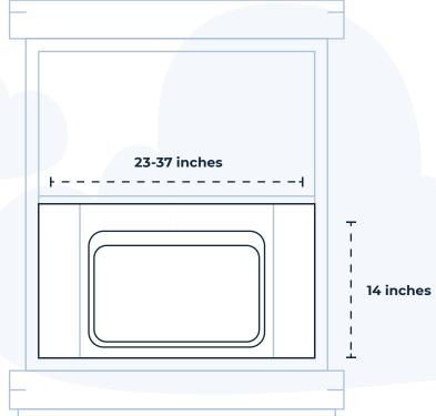
The Windmill AC is designed for windows that slide up and down (double-hung windows) with a width of 23-37 inches and a vertical opening of at least 14 inches.
