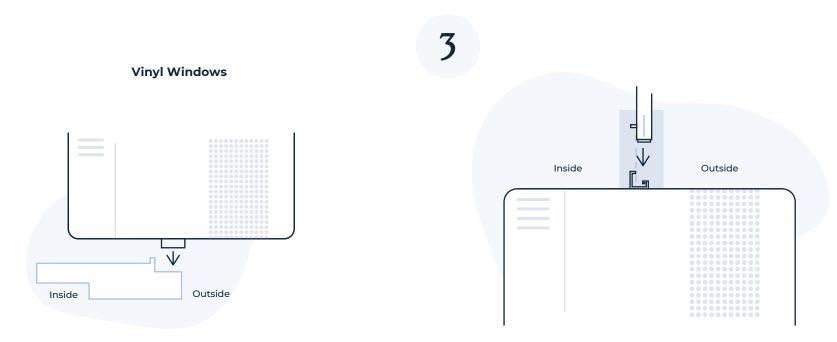
If you have storm windows, additional window setup is required. Otherwise, the unit will tilt into the room (which could damage your floor and the unit). Please visit windmillair.com/support.
