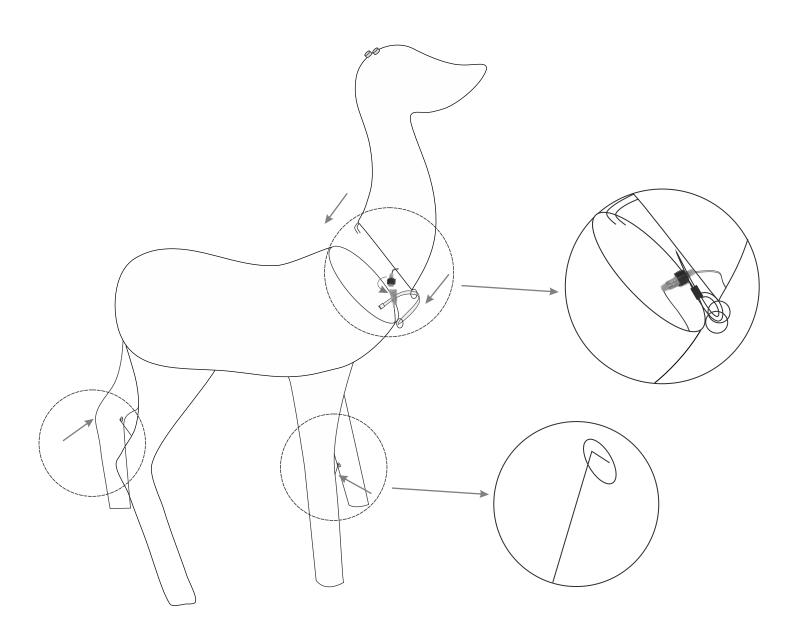
Connect 2 connectors together, use zip tie to connect the deer head with the body, make the 4 feet steady by fixing the wire hook.
