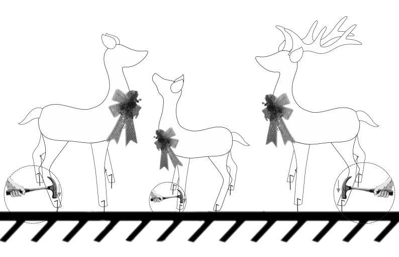
Assembly is now complete, light up with the transformer supplier. If using outdoor on a lawn, secure the deers by inserting the 4 lawn stakes through the supports and into the soil.
