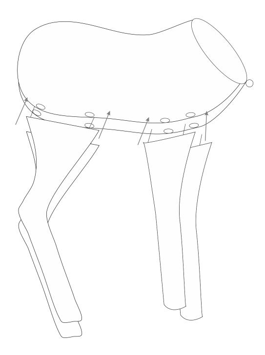
Assemble the deer feet with the body by inserting the wire tubes into the holes located on the body as picture shown.
