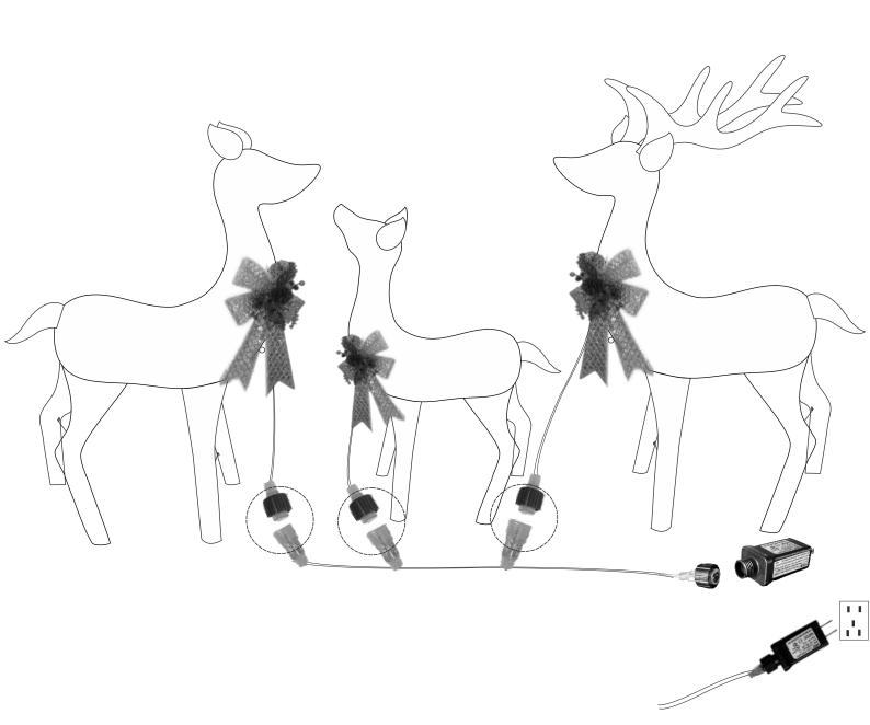
Use the Three-Plugs End Connector to connect three deers cables together, and connect the other end of the connector cable to the transformer.
