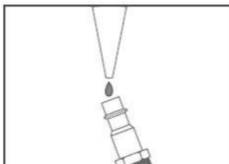
Figure 8. Lubricating stapler via air inlet.
