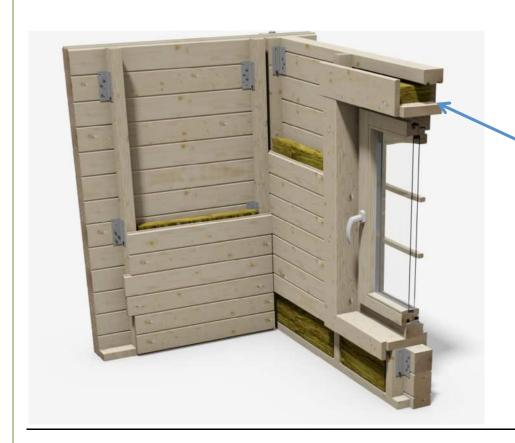
2" of space must be allowed on rough opening at the top of all windows and doors. This cavity is reduced over time as the wall logs settle. Larger trim boards are used on the outside and inside.
