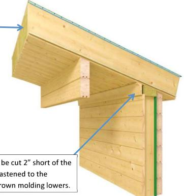
Interior wall cover boards must be cut 2" short of the ceiling and a crown molding is fastened to the ceiling. As the wall settles the crown molding lowers.
