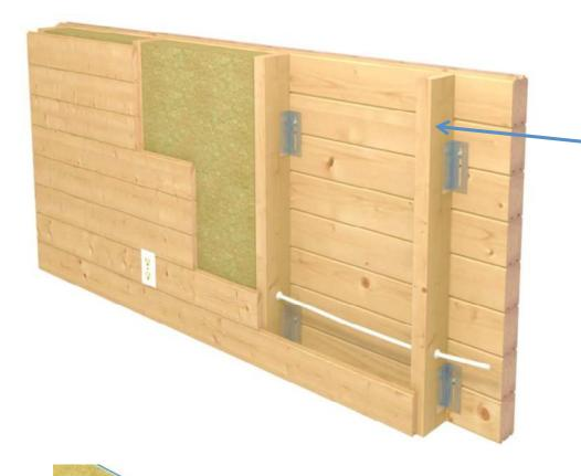
Studs with a depth required for the insulation being used, are installed 16" or 24" on center. Metal brackets are provided to attach the studs to the wall logs. No top plate or bottom plate is required. The metal brackets are designed to allow the exterior wall logs to settle while the studs remain stationary
