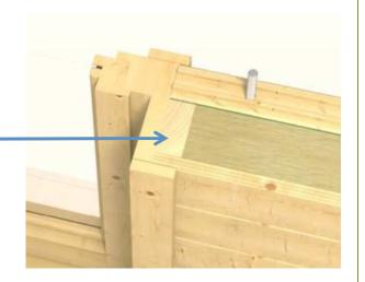
This spacer block is equal to the depth of the studs being used and is sealed and fastened to the bottom and sides of window jambs and sides only of door jambs. (DO NOT apply to the top of jambs)
