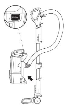
Press Lift-Away™ button to lift pod off motorized floor nozzle.
