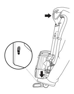
Plug power cord into outlet. Place foot on floor nozzle and tilt handle back.
