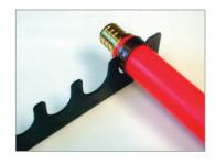
Slide the correct slot on the gauge around the crimped ring.
