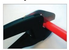
1. Cut tubing end squarely. Check for and remove any burrs.
