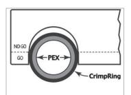
3. If the ring slides into the slot and stops in the "Go" range at least at one point, then the crimp is good. The ring will not fit the go range all the way around it.
