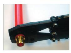
3. Place the crimping end of tool around the crimp ring and press the handles together.
