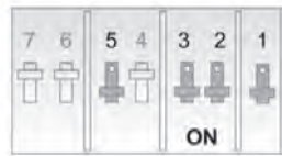
- Dip Switch Detail (Factory Setting Shown)
