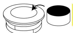
5 - Insert the steel ring on top of the sand. The metal ring should be high enough to protect the inside of the top caps (flush to the top of the caps). If it is not high enough, be sure to build up the base layer inside the center of the firepit to raise the ring higher.
