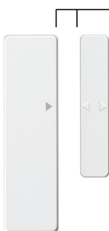
**Gap - less than 3/4" when installed.**
