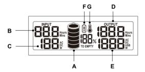
• **A-Battery Level:** The battery level is provided by the percentage of battery charge corresponding to the number of bars and percentage displayed.
