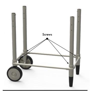
**STEP 4.** Affix VERTICAL TUBES to LOWER CART TUBE ASSEMBLY using provided hex screws and 4mm hex wrench. **Do not fully tighten hex screws at this step.**
