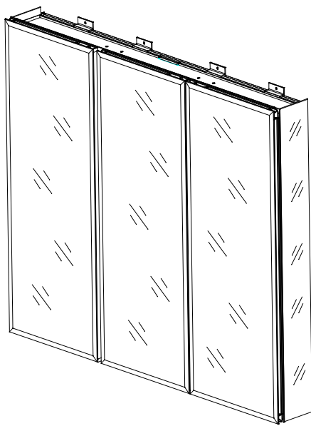
SURFACE MOUNTED CABINET SHOWN
