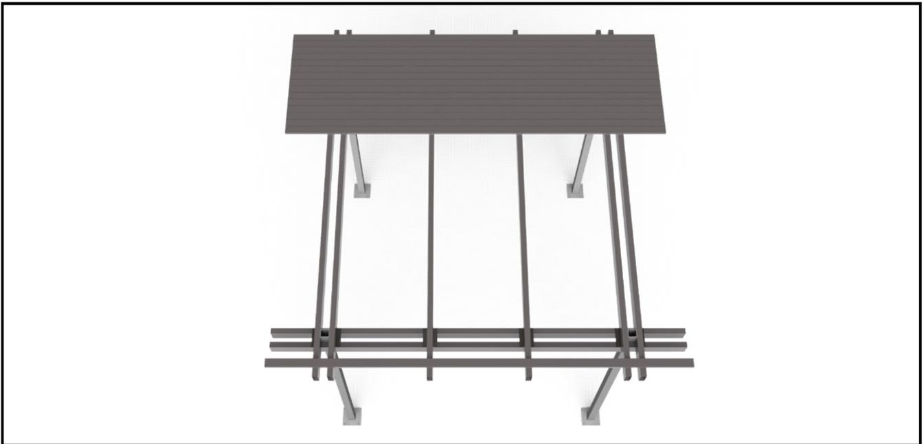
4. The spacing between the shade slats is the width of 2 slats (6 inches). Therefore, leave two and fasten the third shade slat to every rafter using one #10 TEK screw. **(Image 34).**
