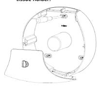
Turn the 3 screws with screwdriver into the plastic plugs and fix the tissue holder on the wall tightly. 4. Drill the holes and insert the plastic plugs into the holes.
