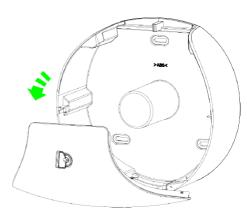
Turn the key by following the direction marked on the keyhole to open the front cover of tissue holder by downward.
