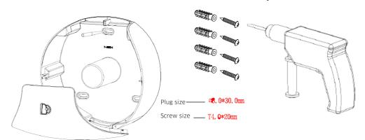
Mark the 3 drilling holes on the wall according to the mounting holes on the bottom shell of the tissue holder.
