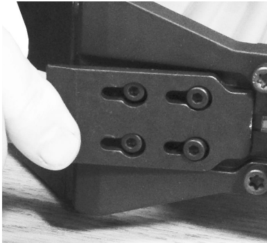
Step 3. Clear drive blade path and reassemble.
