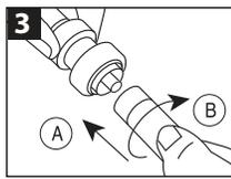
Push pipe (A) and twist (B) into fitting until fitting edge meets depth line.
