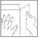
Snap board along the score Using utility knife, cut over the edge of a solid support. (A quick action produces the best results.)
