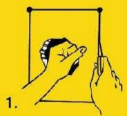
Draw pencil outline around the area to be removed. Cut along line and remove cut out piece.
