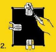
Place Repair Clips 6" apart around the hole. Secure with screws 3/4" from the hole edge.
