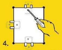
Screw through the patch into Repair Clips. Place screws 3/4" from the edge of the patch.
