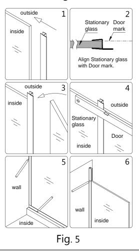
Remove the U-channel 1 (76", wall profile) (09), U-channel 2 (44", bottom profile) (29) and Anti-Water strip (inline panel) (19) from the Stationary glass (11) and set the Stationary glass aside.
