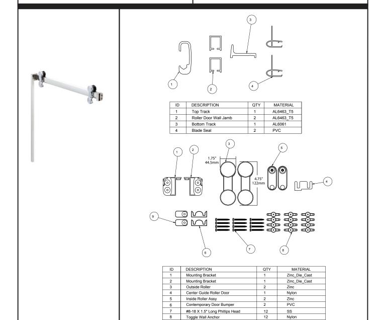
MATERIALS: Anodized Aluminum Excursions (Track) and Zinc Die Cast (Mounting Brackets). Bronze Finish is Powder Coated.
