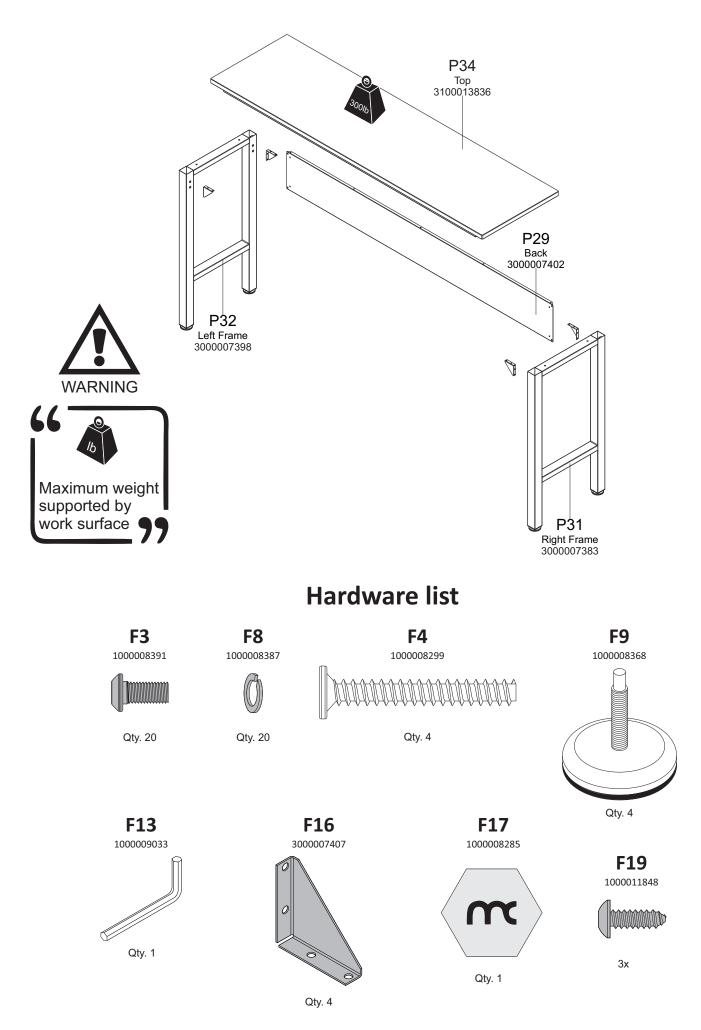
**STEP 1** 1.Fit the shoes to frame **P32** and **P31** base and turn to screw. To level the height or the table, turn the shoe clockwise or counterclockwise until is aligned
