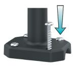
2. Mount the Mast to a flat surface with the four provided screws.
