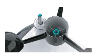
1. Remove the Glide Sensor, Wind Cups, and Mini Screwdriver from the package. Take note of the flat edges located on the head of the Glide Sensor and underside of the Wind Cups.
