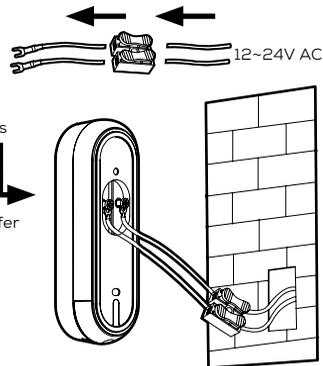
Either wire can be connected to either terminal
